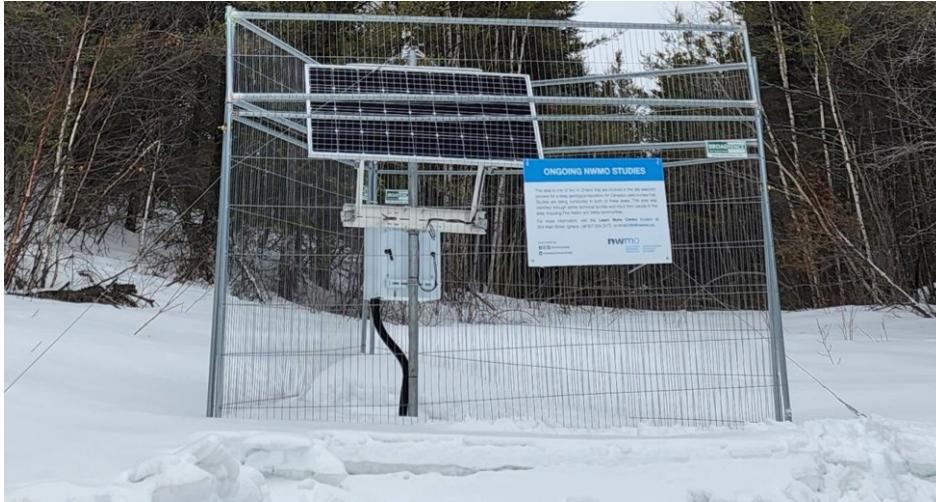
A microseismic station gathers information to further understand the potential for earthquake activity in one of our potential siting communities.
